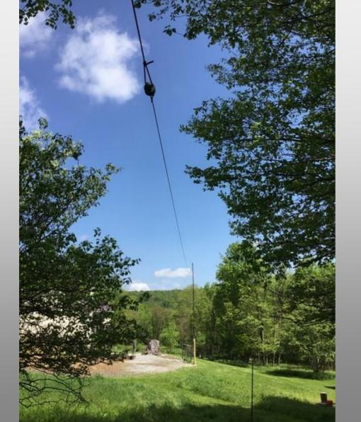
The dipole is 264' long 14 guage PVC coated wire. The center piece used to be one of my wife's cutting boards.
