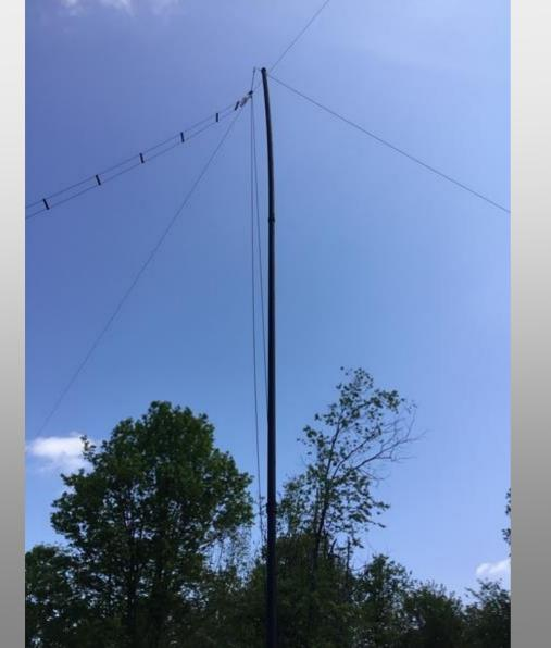
Two 1  $\frac{1}{2}$ " 10' sections of iron pipe topped with one 1 ½" 10' section of PVC. Top has cap and eye bolt to act as "pulley" for antenna maintenance
