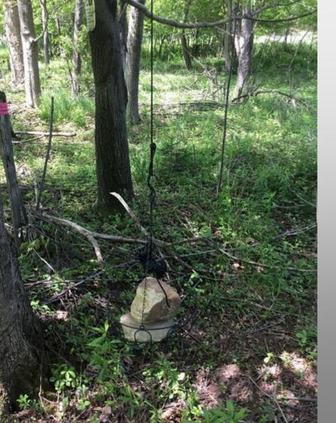
Each end of the dipole runs through a pulley in a tree, and the end is tied to a metal flower basket holding rocks. In the summer, the counterweight is set to be close to the ground.
